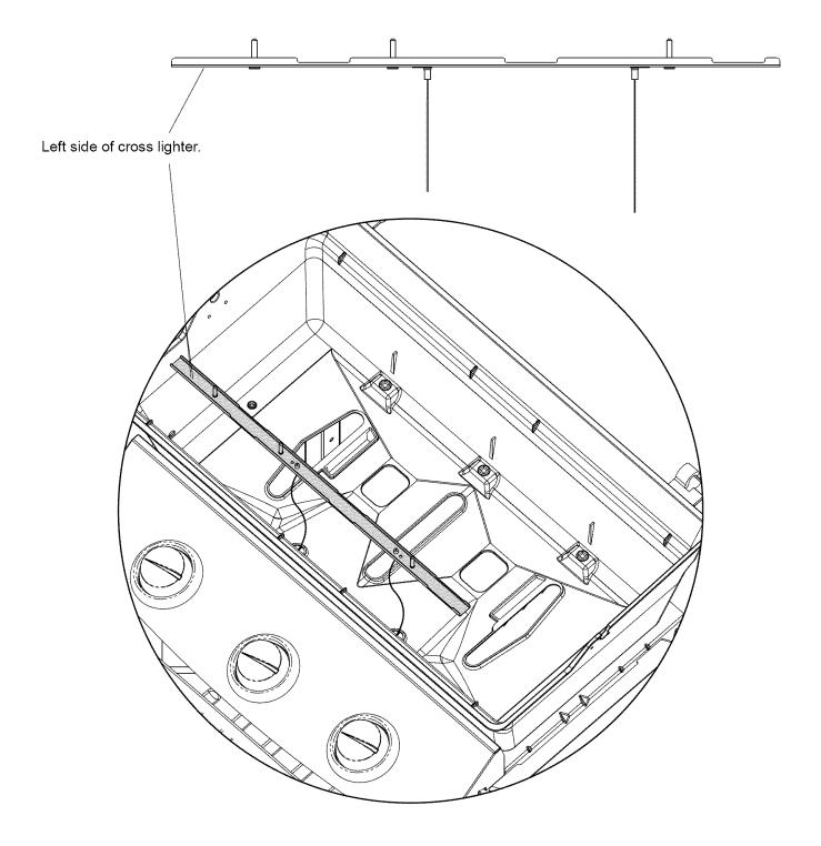
27. Install burners by feeding burner though slot in the base casting and guiding burner tube over orifice in valve, see illustration below. Secure burners with three 1/4"-20 x 3/4" carriage bolts and 1/4"-20 Knurl nuts.
